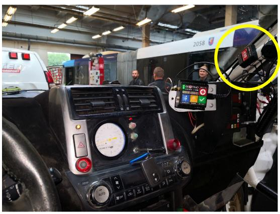
Installation of the GPS TRACKER on the roll cage "A-pillar" of a Car using cable ties.
