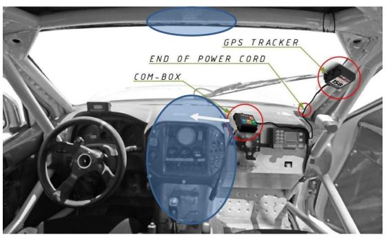
Following a change in the regulations, the '**Com-box'** must be mounted in a central location as per indicated areas in blue, to enable both driver & co-driver to be able to reach the SOS button from their seat with seatbelts on. Shown are the mounting positions of the system components.
