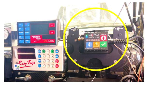
Installation of the Com-Box unit with bracket on the dashboard using bolts. **This must be in a CENTRAL** Iocation and not as indicated above, only in front of the co-driver.
