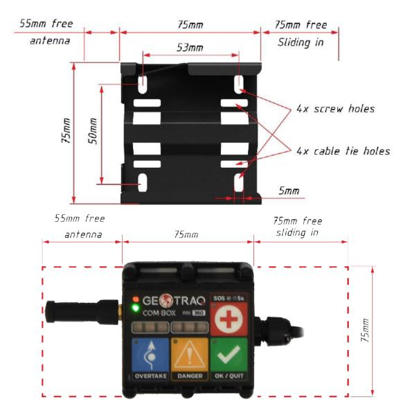
IMPORTANT! No bolt/screw heads or cable/zip ties can protrude over the red line as marked bellow.
